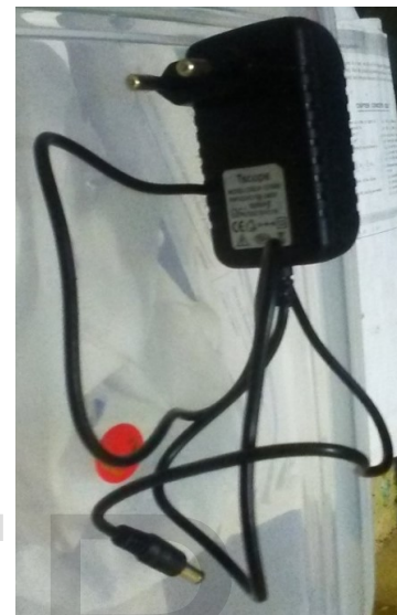
Figure 5: 12V adapter for GSM Modem
